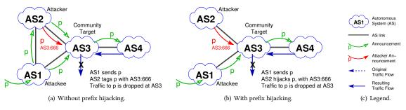
Figure 7: Remotely triggered blackholing.
