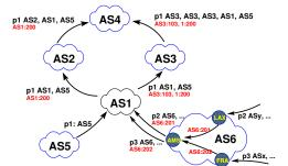
Figure 1: Policies with BGP communities: AS1 requests path prepending by tagging AS3: 103 towards AS3, and informs its peers that prefix p1 is a customer prefix, by attaching community AS1:200. At the same time AS6 uses communities AS6:201 and AS6:202 to signal where a route is learned.
