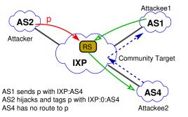
Figure 9: Route manipulation at an IXP with hijacking.
